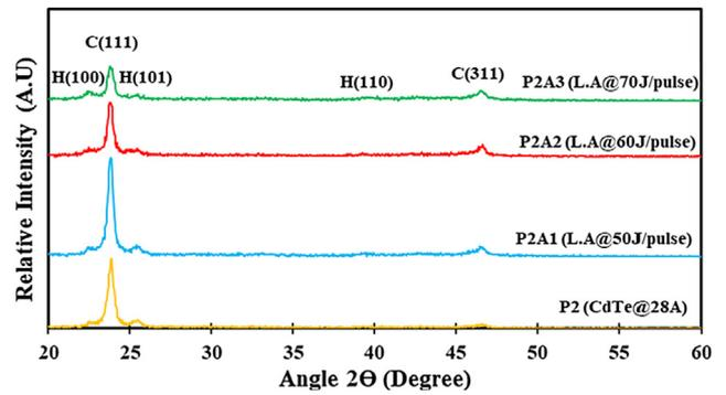
Fig. 1. XRD pattern of as-grown and laser annealed CdTe thin films.
