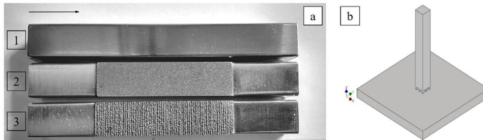
Fig. 1. (a) Photograph of the bending fatigue specimens in different surface conditions. 1: machined specimen, 2: as-built SLM specimen, 3: as-built EBM specimen. (b) Schematic image of one of the bars on a build plate. Arrows in the images indicate the build direction.
