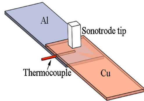
Fig. 2. A schematic for interface temperature measurement.
