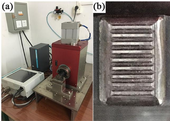
Fig. 1. (a) USW system used in this work and (b) knurl pattern of sonotrode.
