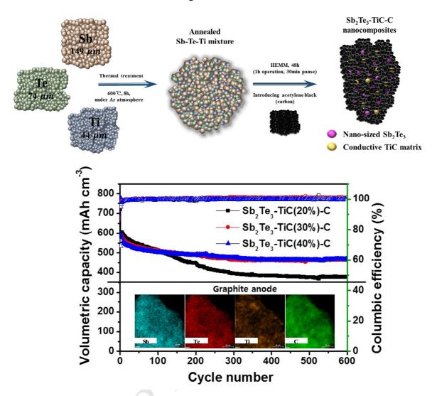
Nanocomposite of  $Sb_2Te_3$ -TiC-C is synthesized via a simple and scalable high-energy mechanical milling process and heat treatment as a high-performance anode material for lithium-ion batteries. The appropriate amount of TiC formation into  $Sb_2Te_3$ -C significantly improves the electrochemical performances.
