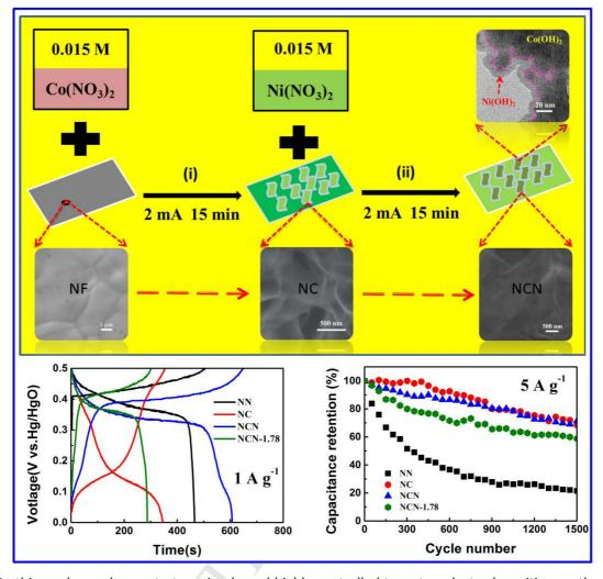
In this work, we demonstrate a simple and highly controlled two-step electrodeposition method for construction of cobalt hydroxide @nickel hydroxide core-shell heterostructure that are directly grown on conductive substrates, which shows better electrochemical performance than its single component counterparts.
