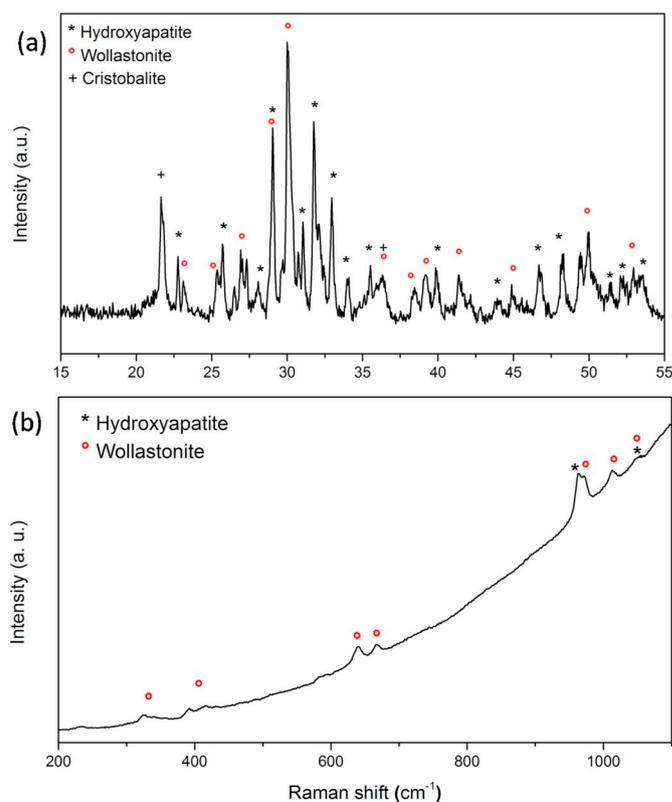
Fig. 1. XRD pattern (a) and Raman spectrum (b) of RKKP-Mn target material.
