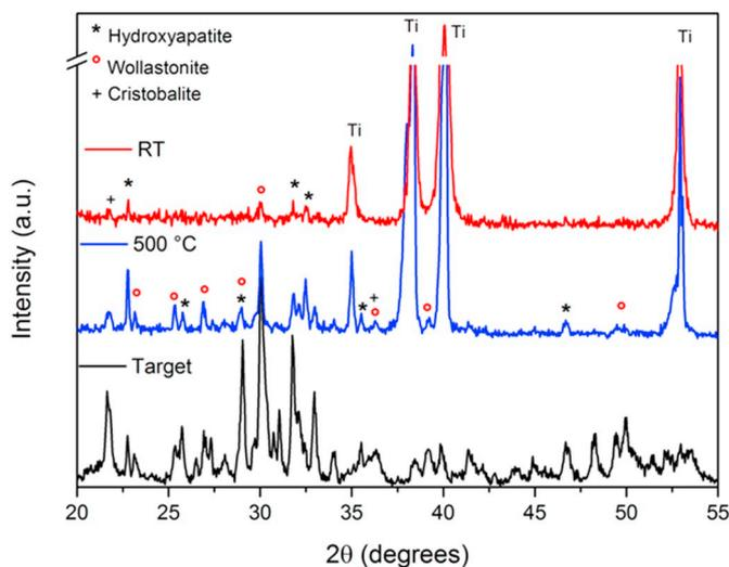
Fig. 2. XRD patterns of RKKP-Mn films deposited on Ti at RT and  $500^\circ\text{C}$ , compared to the target one.
