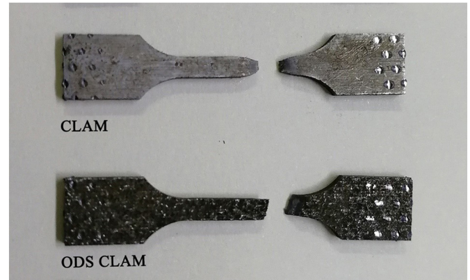
Fig. 2. Tensile sample size and appearance of ODS CLAM specimens.
