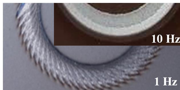
Fig. 1. Visual comparison of the silicon target surface for 1 and Hz laser shot repetition rates.
