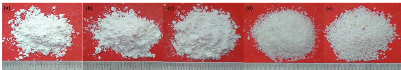
Fig. 1. Calcium carbonate material with various size ranges ((a) CaCO 3 -1; (b) CaCO 3 -2; (c) CaCO 3 -3; (d) CaCO 3 -4 (e) CaCO 3 -5).
