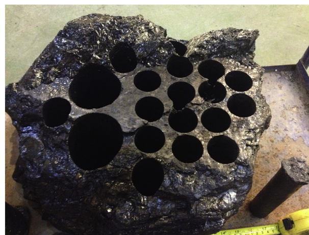
Fig. 2. A typical coal block used for the extraction of coal samples for uniaxial compressive tests.
