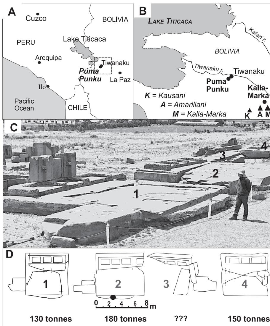
**Fig. 1.** (A) South American Andes with Pumapunku/Tiwanaku. (B) Location of the geological sites selected in this study. (C) The 4 megalithic red sandstone slabs of Pumapunku. (D) Drawing and dimensions of the 4 slabs.
