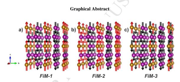
Ferrimagnetic configurations considered to obtain the Fe-Mn (FiM-1), Mn-Mn (FiM-2) and Mn-Fe (FiM-3) exchange coupling constants in FeMnO<sub>3</sub> material. Purple, orange and red balls correspond to Mn, Fe and O atoms; respectively. Red and Black vectors represent spin up and down, respectively.
