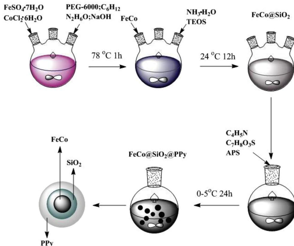
Fig. 1. Schematic demonstration of the FeCo@SiO<sub>2</sub>@PPy ternary composites.
