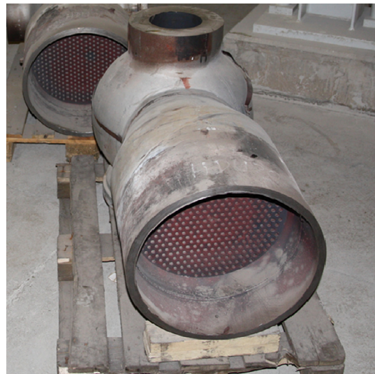
Fig. 1. Turbine bypass valve (fabricator: Bopp & Reuther) [1].
