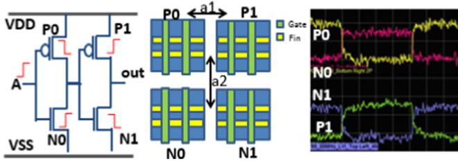
Fig. 1. Layout and schematic of an inverter LVP waveforms show that the phase of the signal on each adjacent transistor (P0, N0), (P0, P1), (N0, N1), (P1, N1) is opposite of each other.
