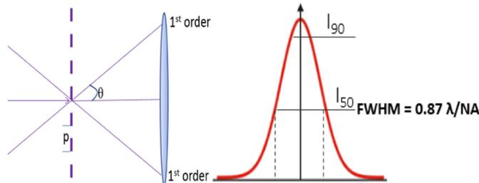
Fig. 2. Spatial resolution can be understood as being able to collect at least 1 diffraction order from a sinusoidal grating with spatial period  $p$ . The  $NA$  of the lens and the wavelength determine the numerical value of  $p$ . Conversely, the laser probe can be pictured as a Gaussian distribution as on the right as well.
