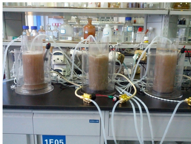
Fig. 1. Set up of autotrophic, heterotrophic and mix-trophic reactor.
