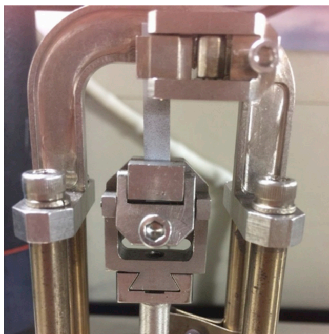
Fig. 3. A sample in tensile clamp.
