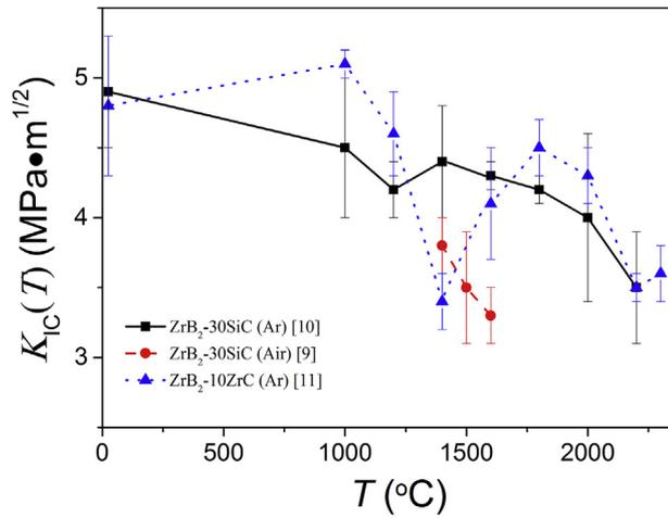
Fig. 1. The existing experimental measurements of fracture toughness of pUHTCs at elevated temperatures [9–11].
