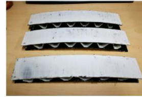
Fig. 1. The fabrication of two kinds of curved beams. (a) The process parameters of hot-pressing. (b) Molds. (c) Hot-pressing. (d) Fabricated specimens.
