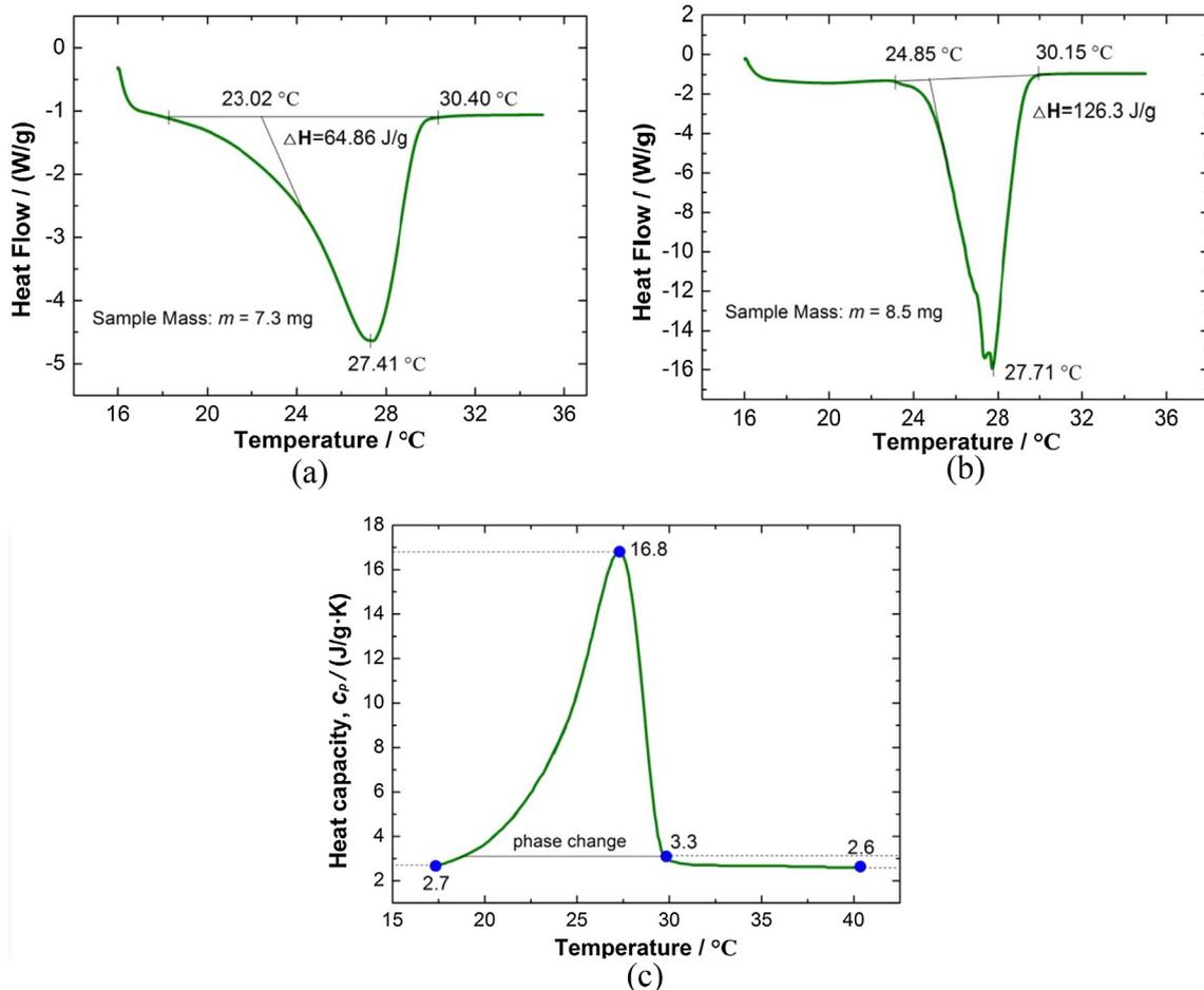
Fig. 1. DSC measurements of thermal properties; (a) Melting points and latent heat of MEPCM; (b) Melting points and latent heat of core PCM; (c) heat capacity of MEPCM.
