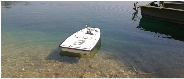
Fig. 1. Mobile platform that we used: Platypus Lutra equipped with pH, Dissolved oxygen, temperature and electrical conductivity sensors. The computation is on board and performed by an Arduino Due and a smartphone.
