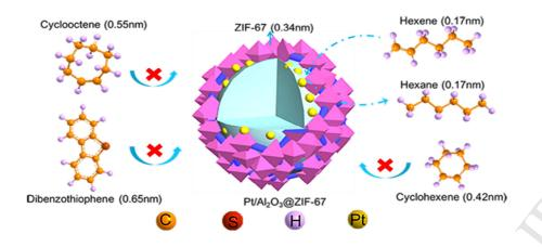
A new core-shell catalyst was prepared by coating a platinum/alumina ( $Pt/Al_2O_3$ ) core with a ZIF-67 shell membrane. The  $Pt/Al_2O_3$ @ZIF-67 catalyst exhibited excellent hydrogenation selectivity, long term stability and sulfur resistance.
