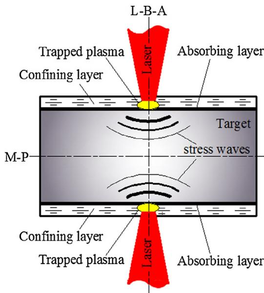
Fig. 1. Schematic of TSLSP (L-B-A represents the laser beam axis, and M-P denotes the mid-plane).
