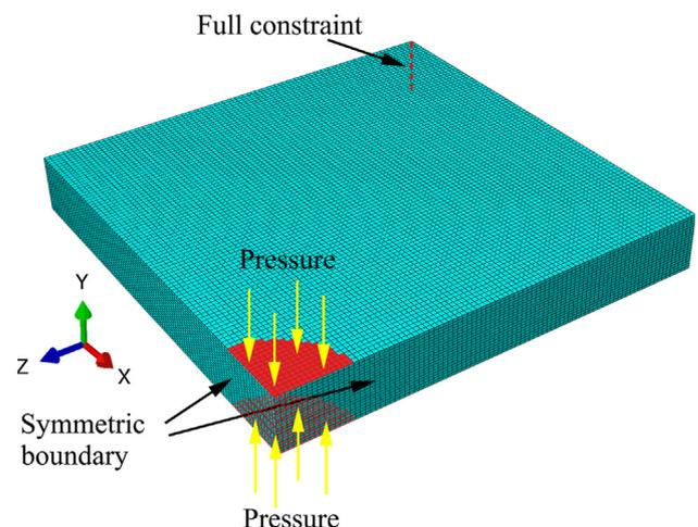
Fig. 2. Schematic of three-dimensional quarter model for TSLSP.
