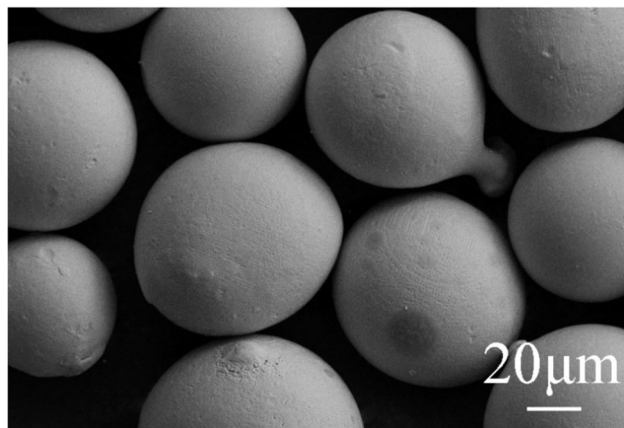
Fig. 1. Morphology of the 316ss powders.
