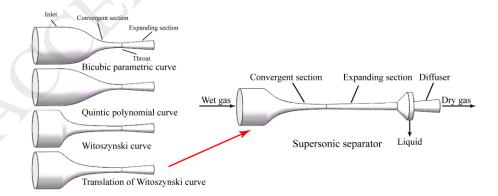
The numerical simulations of CH<sub>4</sub>-CO<sub>2</sub> mixture gas in the nozzle were carried out applying User Define Function, which convergent section is designed by different
