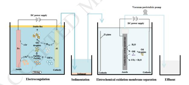
Abstract: A novel electrocoagulation (EC)-carbon membrane coupling with electrochemical anodic oxidation (CM/EAO)
