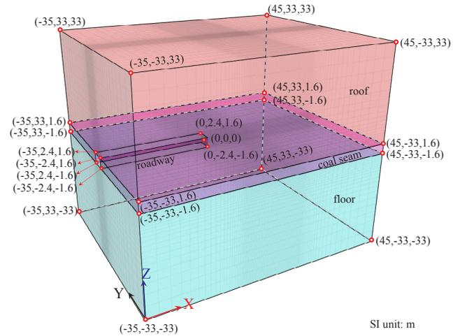
Fig. 1. Numerical calculation model and the key point coordinates (SI unit: m).
