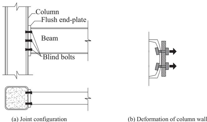
Fig. 2. CFST column endplate joints with blind bolts.
