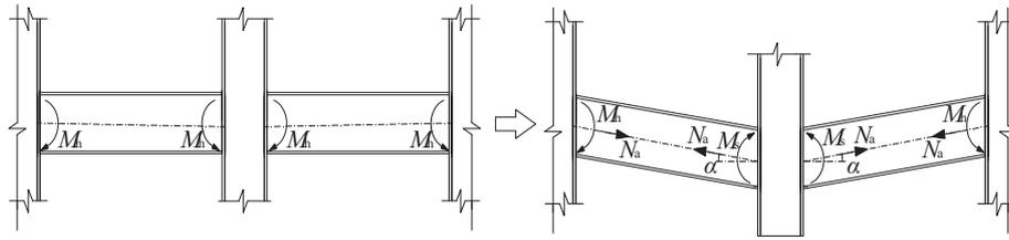
Fig. 1. Load-carrying action transition.
