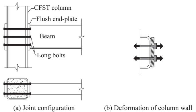
Fig. 3. CFST column endplate joints with long bolts.
