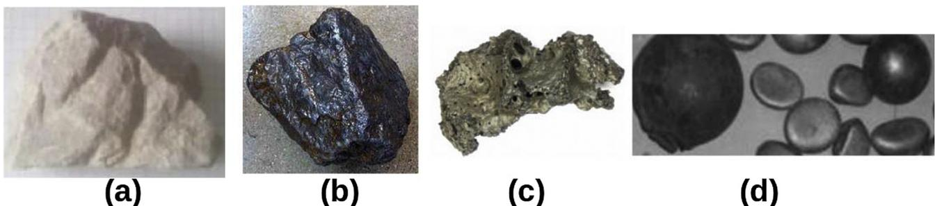
Fig. 1. (a)–(c) Shape of typical material in mills, (d) new and worn balls from a ball mill.
