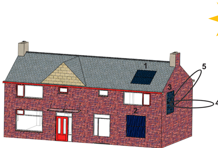
1,2,3: Solar panels 4: Reception pattern of the solar panel 3 without ARC 5: Reception pattern of the solar panel 3 with ARC
