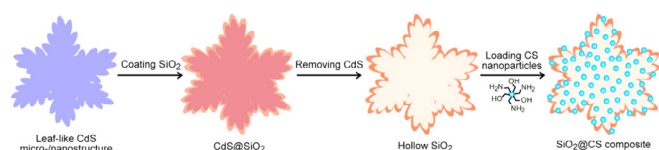
Fig. 1. Illustration for the preparation of the SiO_2@CS composite with a biomimetic leaf-like structure.
