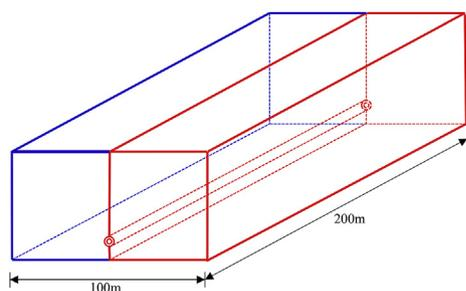
Fig. 1. A representative model for cyclic steam stimulation using single horizontal well with only half of the model (right zone in red) used for numerical simulation owing to symmetry. (For interpretation of the references to colour in this figure legend, the reader is referred to the Web version of this article.)
