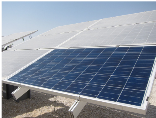
Fig. 1. Soiled and cleaned PV modules after one month of soiling at the QEERI Solar Test Facility in Doha, Qatar.
