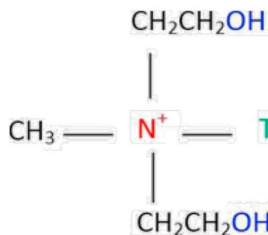
Fig. 1. The structure of modifier in Cloisite30b (T:tallow is carbon chains consist of 65% C18, 30% C16, 5% C14) (Kotal and Bhowmick, 2015).
