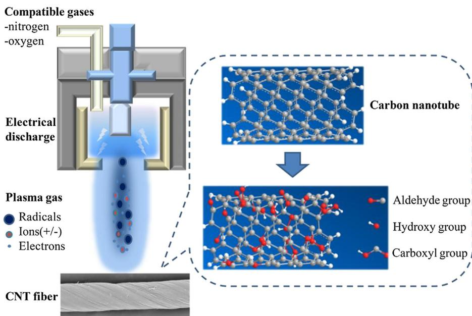
Fig. 1. Schematic showing the atmospheric pressure plasma treatment on the CNT fiber.
