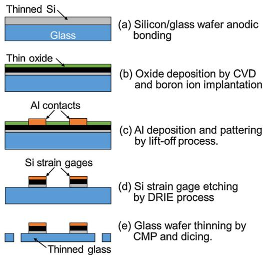
**Fig. 1.** Schematic depiction of fabrication sequence for silicon strain gages onto glass substrates.
