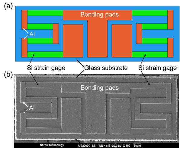
**Fig. 2.** Silicon strain gage on glass substrate: (a) layout and (b) SEM.
