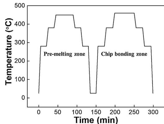
**Fig. 3.** Pre-melting and bonding profiles of screen-printed glass-frit on metal diaphragm.
