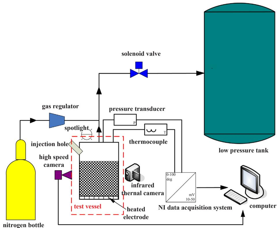
Fig. 1. Schematic diagram of experimental system.
