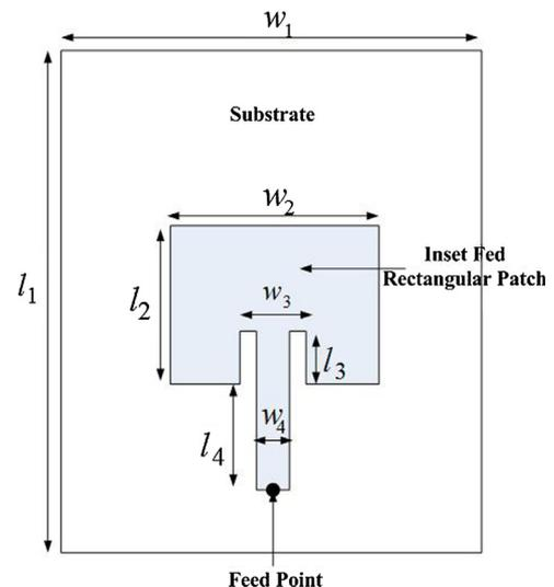
Fig. 2. Structure of inset fed rectangular patch antenna for 5 GHz and 5.9 GHz.
