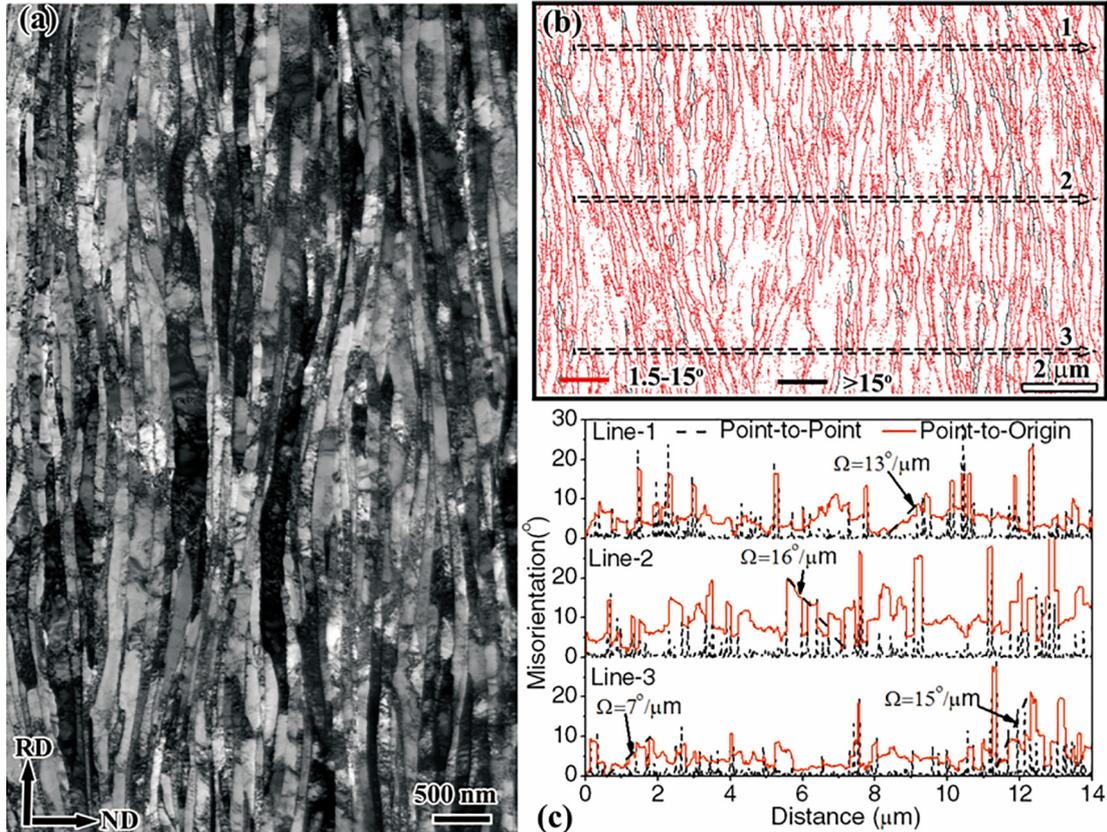
**Fig. 1.** Deformation microstructure of Brass-oriented single crystal Ni: (a) TEM image, (b) a boundary map reconstructed from EBSD data, and (c) the variation of the misorientation (point-to-point and point to origin) as a function of distance along the three lines parallel with ND in (b). (For interpretation of the references to color in this figure, the reader is referred to the web version of this article.)
