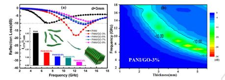
By controlling the content of GO, the average conjugation length of PANI nanorods on GO layers can be modulated, resulting in controllable wave-absorbing properties and various frequency bands.
