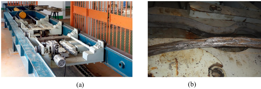
Fig. 1. a) Horizontal online tensile testing machine and b) crushed surface of a steel wire rope.
