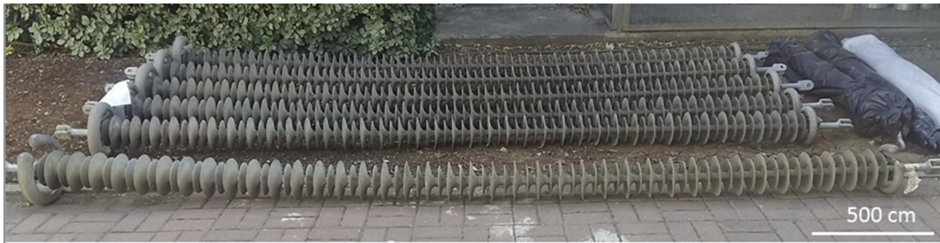
Fig. 1. 400 kV composite insulators (Reliable corp.)
