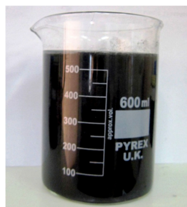
Fig. 2. Nanofluid obtained by suspension of functionalized multi-walled carbon nanotubes in a mixture of water and ethylene glycol.
