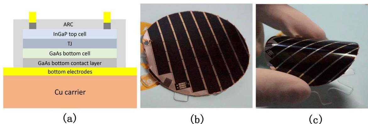
Fig. 1. (a) Schematic diagram of the fabricated InGaP/GaAs double junction TFSC device. (b) Photograph of a 2-in. TFSC wafer on a plane in natural state and (c) Photograph of a 2-in. TFSC wafer in bending state.
