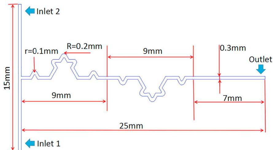
Fig. 2. The planar dimensions of the micromixer.
