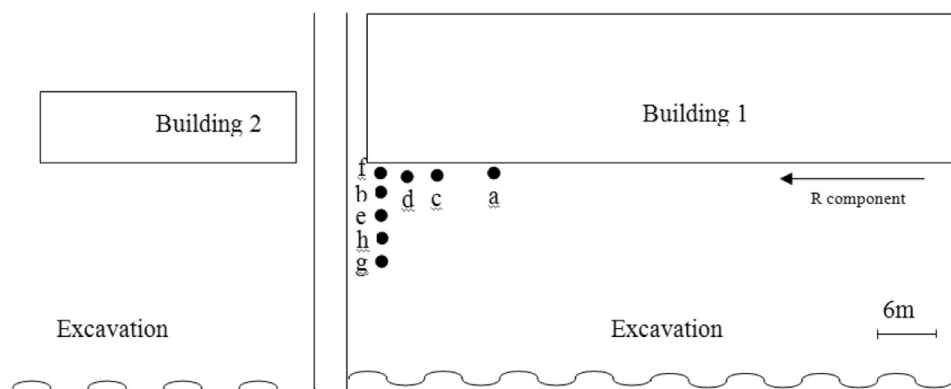
Fig. 1. Blast locations shown with respect to the buildings. As can be seen from the scale, fragmentation of rock was required immediately adjacent, or contiguously, to the buildings (shots f, d, c & a), which produced the ultra-high frequency excitation motions.
