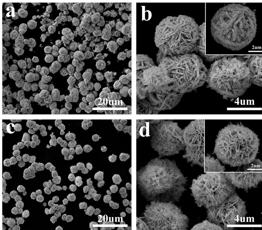
**Fig. 1.** SEM images of samples prepared with different acid at  $160^\circ\text{C}$  for 24 h. (a, b) nitric acid, S1; (c, d) acetic acid, S2. The insets are the corresponding SEM images with high magnification.
