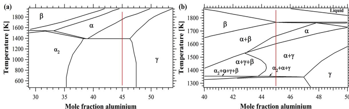
Fig. 1. (a) Binary phase diagram of Ti-Al [18]; (b) Section through a proposed phase diagram of the Ti-Al-Nb alloy system for an alloy containing 7.5 at. % Nb [19].
