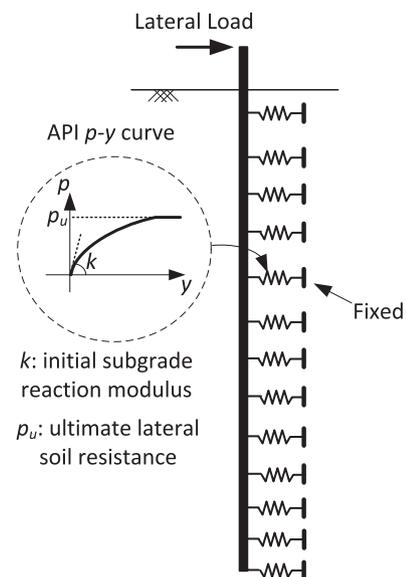
**Fig. 1.** Schematic of the spring method used in practice for static analysis of laterally loaded single piles.
