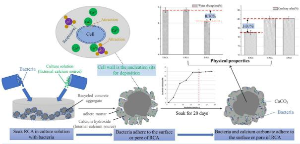
Note: bacteria can obtain calcium source from culture solution(external calcium source) and adhere mortars(internal calcium source).
